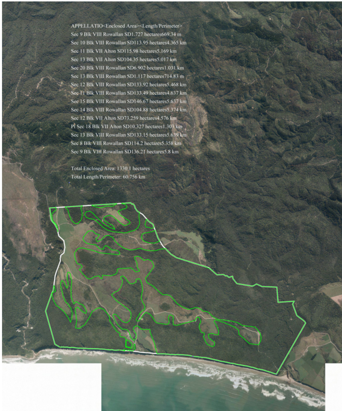
Figure 2.3.5e. 1990 Eligibility Map. Green lines demarcate the forest/non-forest boundary as of 1990. Resolution for aerial image for 1990 forest/non-forest boundary: 30m. Image date for backdrop photo: March 2011.
